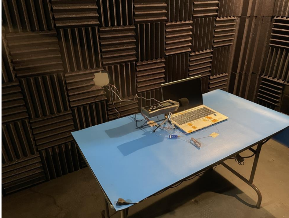
Figure 13. HP EliteBook 840 G8 shown inside of the STL pseudo-anechoic chamber.
